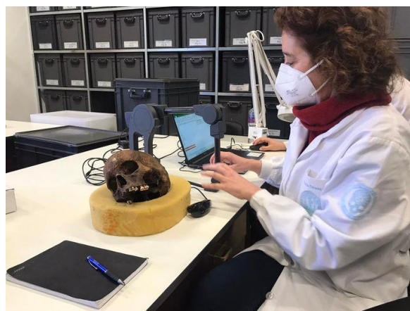
Figure 19 - MicroScribe® G2X data acquisition. Equipment is set on a stable workbench and the specimen fix in a proper support.
