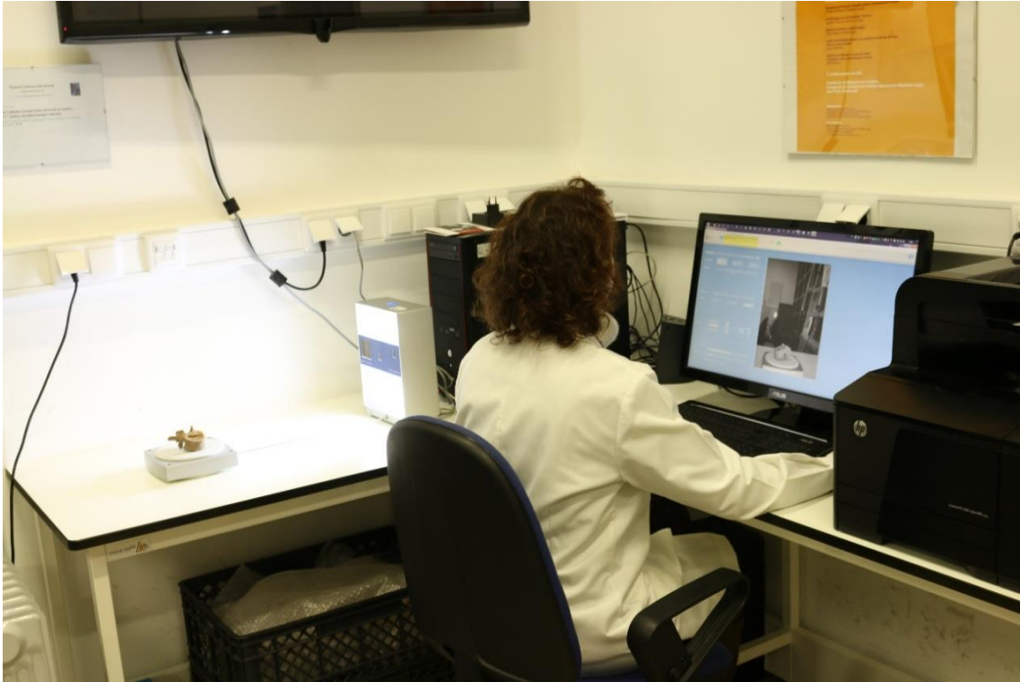
Figure 18 - Beginning of 3D acquisition. The hardware is set on a workbench, with the sample in the turntable. On the computer screen, the scan settings dialog box is visible (the settings are on the left; the camera viewport is on the right).
